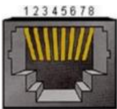
RJ45 connector pin number definition (top view)
